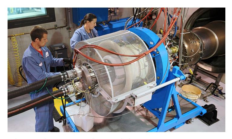
With two comprehensive engine test cells on-site, Columbia Helicopters is capable of providing engine MRO services to numbers engines and APUs. Columbia is a factory-authorized service center for the Honeywell T55-714 series engine. The facility also maintain a Honeywell correlated test cell capable of operating up to 6,000 shaft horsepower.
